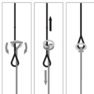
**Step 6:** Pull the HFL Left (red) from the bottom, through the attached O-Ring until the Bullet stopper ball touches the O-Ring.
